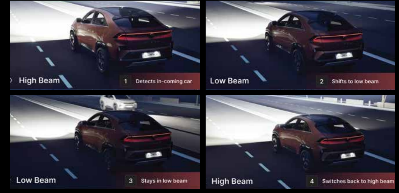
HIGH BEAM ASSIST (HBA) Automatically switch between high and low beams for optimal visibility.
